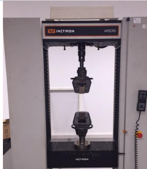
INSTRON4505 cell load capacity of 100kN
