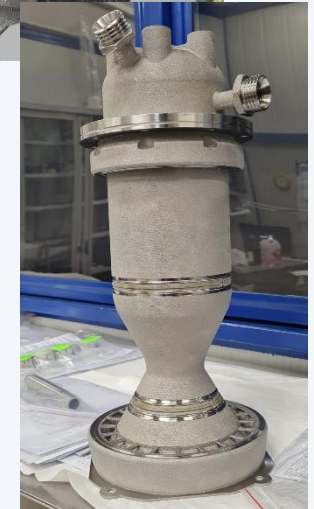
Combustion Chamber mock up
