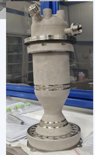
Combustion Chamber mock up
