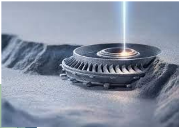
L-PBF: Laser Powder Bed Fusion
