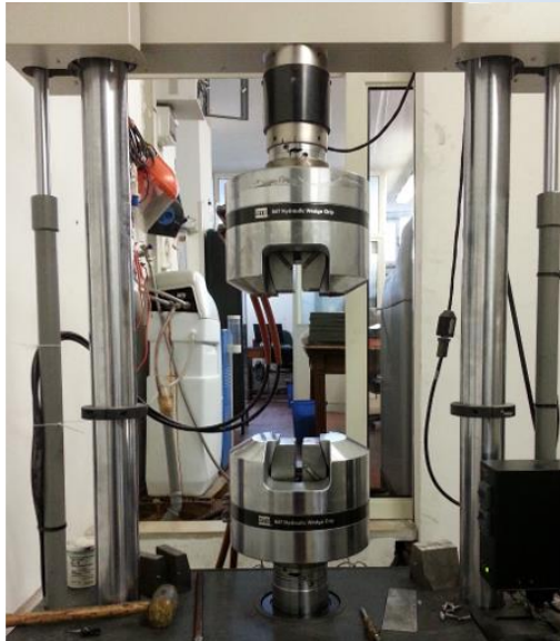
MTS810 cell load capacity of 250kN
