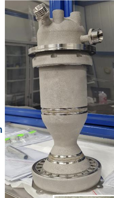
Combustion Chamber mock up
